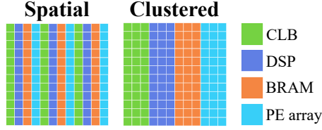
Figure 3: Layout strategies to be explored. Blocks extend vertically in columns and repeat horizontally based on the strategy.
